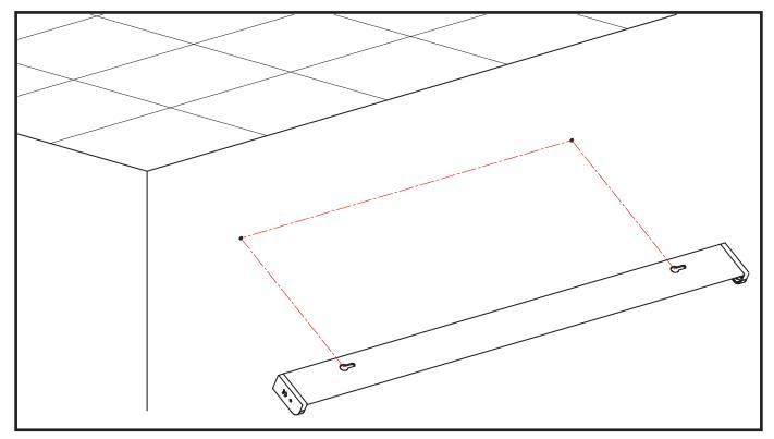
2. Insert a mounting anchor of the proper size and weight rating in each hole, then thread one screw of the proper size and weight rating into each anchor. Please note that mounting hardware is not included. Do not tighten the screws down completely! Leave a gap of approximately 2mm between the mounting surface and the head of each screw.
